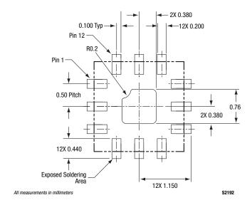
Figure 9. SKY13373-460LF PCB Layout Footprint (Top View)
