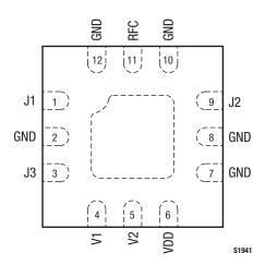
Figure 2. SKY13373-460LF Pinout (Top View)
