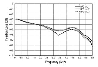
**Figure 3. Typical Insertion Loss vs Frequency**
