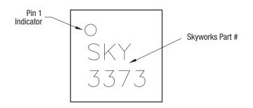
Figure 10. Typical Part Markings (Top View)
