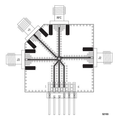
Figure 8. SKY13373-460LF Evaluation Board Assembly Diagram
