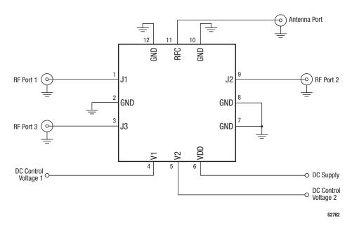
Figure 7. SKY13373-460LF Evaluation Board Schematic
